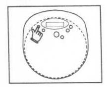
During stop, press PROG button until "PROG " flashes in LCD. The track number and playing order appears.
